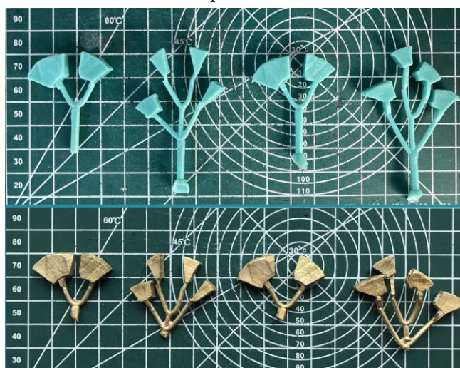
Figure 4. Upper photo with wax moulds before metal casting and lower photo with brass moulds after casting.
