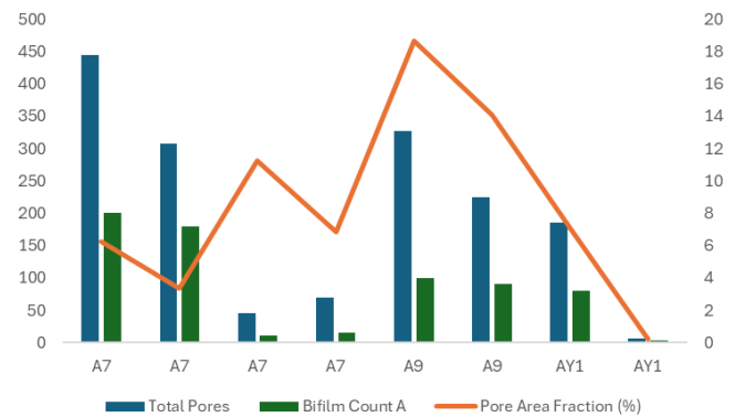
Figure 8. Pore Quantity and Bifilm Calculation Results
